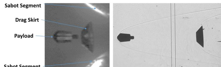
Drag Skirt Separation in Ballistic Range Flight: M = 11.5
