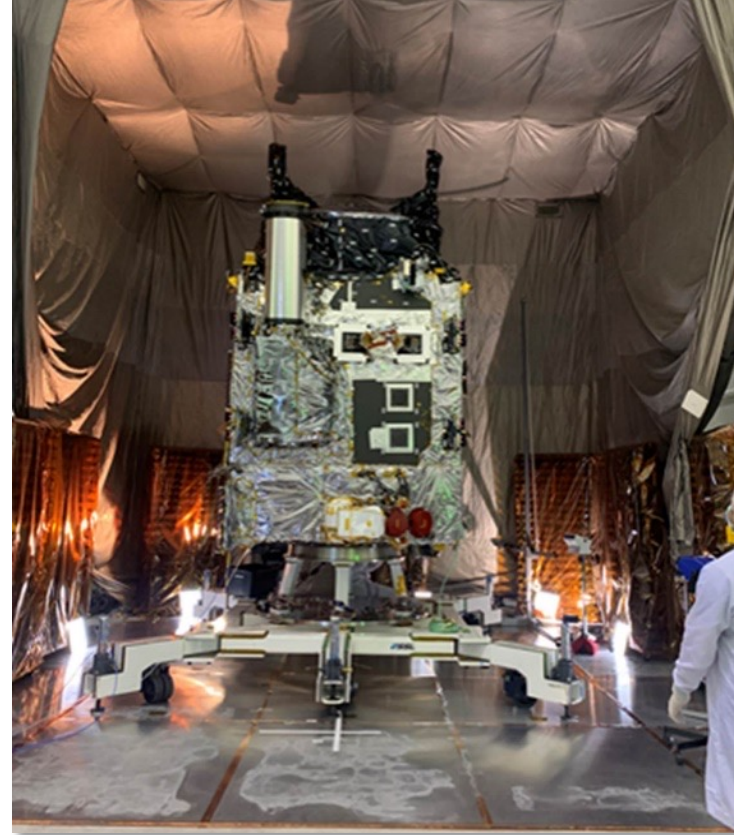
Above: Psyche in EMI/EMC tent Right: Psyche being moved 'up the hill' to TVAC testing
