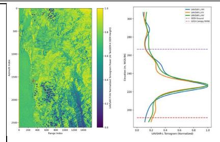
Comparing UAVSAR tomogram power profiles to GEDI data shows complex (multiple peak) structure of tall redwood forests. Example profile has GEDI canopy height of 75 m. Ground peak can be observed at P-band but not L-band
