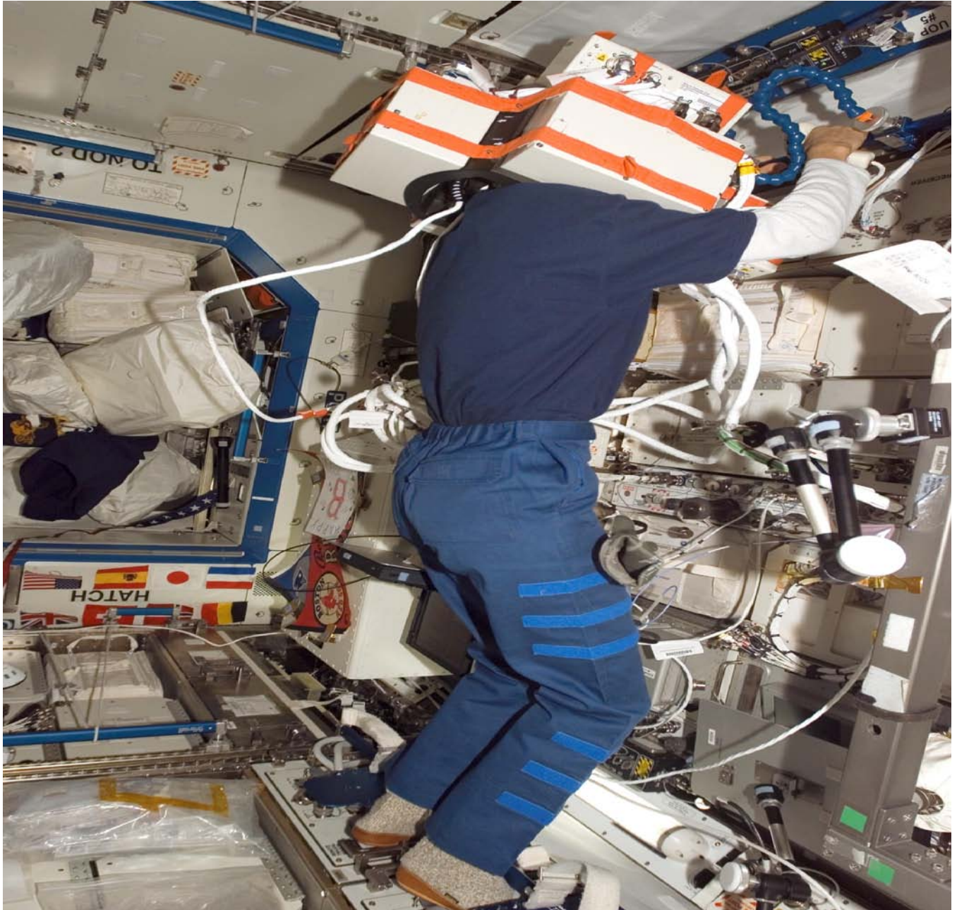
Figure 4. Expedition 13 ISS (International Space Station) Science Officer Jeff Williams shows off Italian cosmic ray detecting headgear. He stayed in the ALTEA helmet for 90 minutes.
