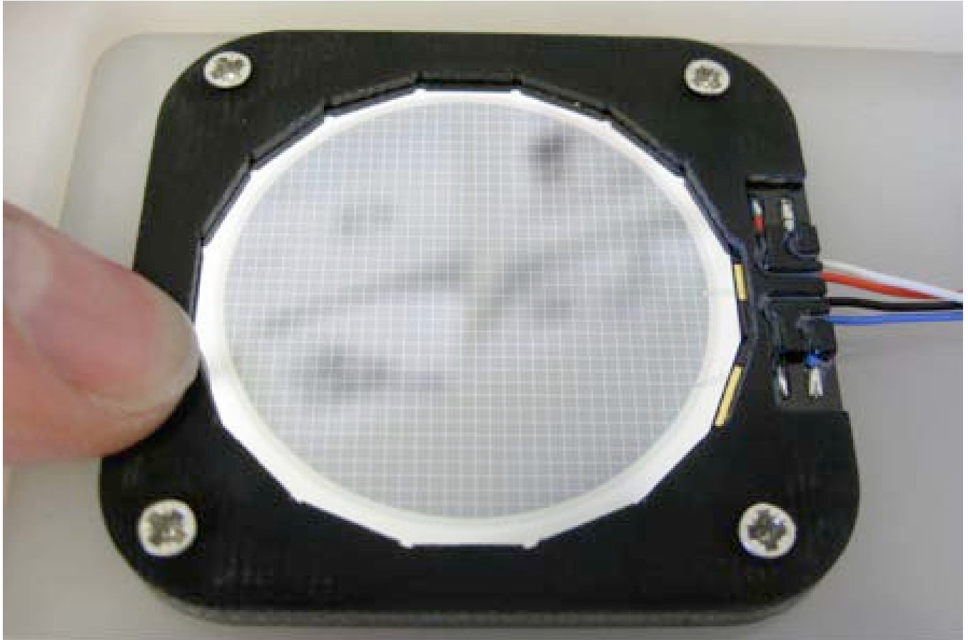
Figure 4. This is an up-close view of a particle detector identical to the six in CRaTER (finger is there for scale). The black plastic frame holds the disk. The disk is 140 micro-meters thick and about 4 cm in diameter. The dark gray squares are the silicon, and the lighter edges of the squares are aluminum. The aluminum improves detecting the current created by cosmic rays. The wires run from the detector to a small computer. The detector is very reflective; in it you can see a fuzzy image of pictures hanging on my office wall.
