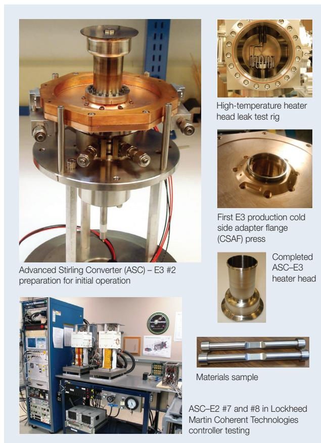
Flight-quality hardware for the first ASRGs is being produced, assembled, and tested in a variety of locations across the country.
