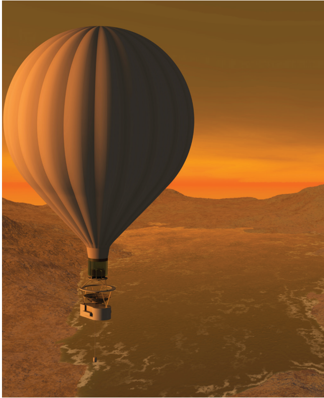
A concept for an RPS-powered hot-air balloon that could explore the atmosphere of Saturn's moon Titan for several months, and perhaps analyze samples of its methane lakes.
