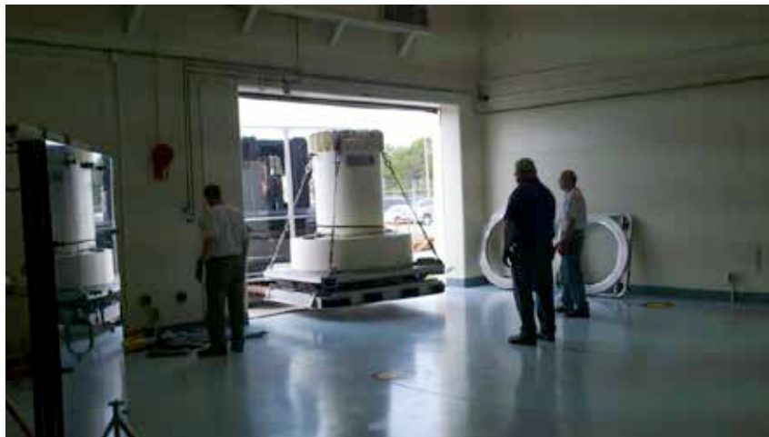
FIGURE 3-27 | 9904 RPS SHIPPING CASK IN RADIOISOTOPE THERMOELECTRIC GENERATOR FACILITY AT KSC
