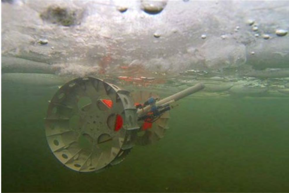
Fig. D-6. BRUIE under ice rover (NASA/JPL).
