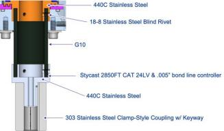
Figure 6: Thermally isolating tool interface. This coupling maintains a >200 K thermal gradient while capable of transmitting over 100 Nm of torque.
