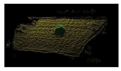
Figure 13: Recognized reference plane (yellow) with segmented sand sample (green)
