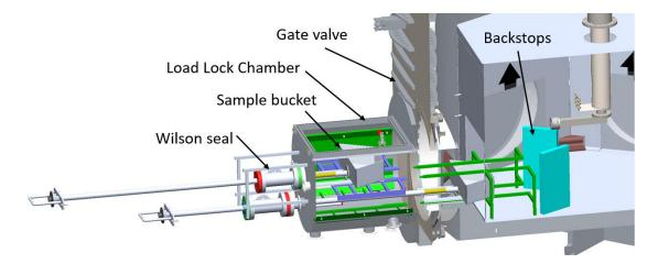
Figure 4: Section view of a load lock with sample buckets (lid not shown). The upper sample bucket is still in the load lock volume while the lower bucket is halfway between the load lock and the backstops.
