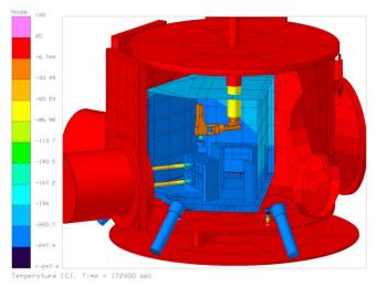
Figure 2: Thermal simulation of CITADEL at steady state cold conditions. The baseplate and sample buckets reach as low as 30 K.
