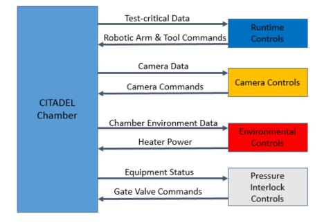
Figure 7: CITADEL Control System Components
