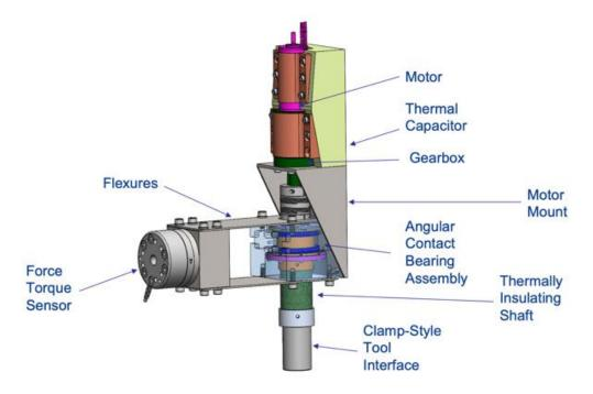
**Figure 5: End effector components**
