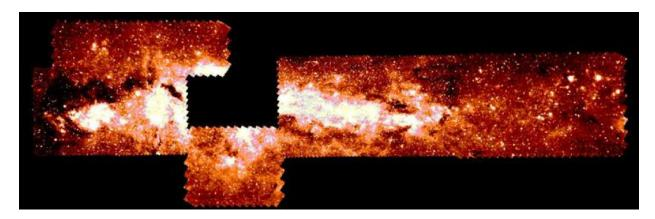
The data your satellite produces might look like real data from the Infrared Space Observatory (ISO), a European satellite launched in 1995. ISO had four instruments, including a camera (ISOCAM), a photometer (ISOPHOT), and two spectrometers (SWS and LWS). This scan across a portion of our Milky Way galaxy was done by the Infrared Space Observatory CAMera (ISOCAM) at an infrared wavelength of 7 microns.
