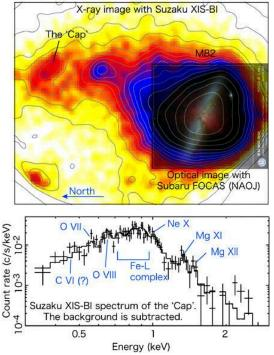
The data your satellite produces might look like this real data from the Suzaku satellite, a joint Japanese-US astronomy mission that was launched in 2005. One of Suzaku's instruments was the X-ray Imaging Spectrometer (XIS), which consisted of four X-ray CCD cameras, each combined with a single X-ray Telescope (XRT).
