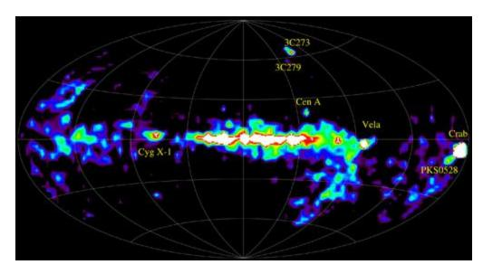
The data your satellite produces might look like this real data from the Imaging Compton Telescope (COMPTEL) instrument that was onboard the Compton Gamma Ray Observatory (CGRO). COMPTEL was the first instrument to survey the entire gamma-ray sky; this all-sky map is the result.
