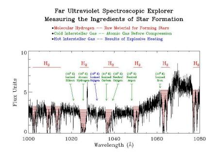
The data your satellite produces might look like this real data from the spectrograph on the Far Ultraviolet Spectroscopic Explorer (FUSE) satellite, which was launched in 1999. The ultraviolet spectrum above, which shows intensity of light over a range of wavelengths, is of a quasar called ESO141-G55.
