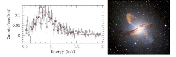
The data your satellite produces might look like this real data from the ACIS instrument on the Chandra satellite. The ACIS is an X-ray imaging spectrometer, which means it has a CCD for imaging but can also measure the spectrum (or intensity over different wavelengths) of a source.
