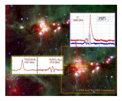
The data your satellite produces might look like this real data from the Heterodyne Instrument for the Far Infrared (HIFI) on the European Space Agency's Herschel satellite, a far-infrared and submillimeter mission that at the time of its launch in 2009, was the largest telescope to be put into space. This spectrum, or graph of intensity over a range of wavelengths, is some of the first data produced by Herschel, and was a test of its capabilities.
