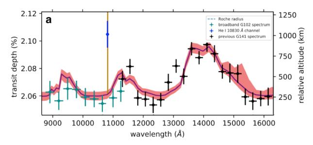
The data your satellite produces might look like this real data, captured by the Wide Field Camera 3 (WFC3) on the Hubble Space Telescope. WFC3 was used in a mode that allows spectroscopy to examine the atmosphere of exoplanet WASP-107b in the infrared.
