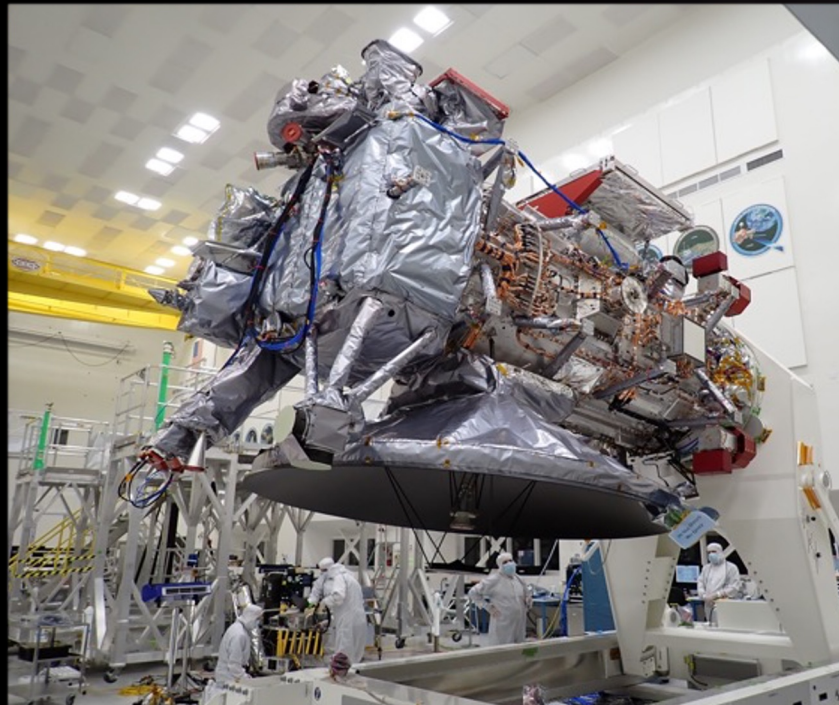
Random vibrate testing (Y axis)
