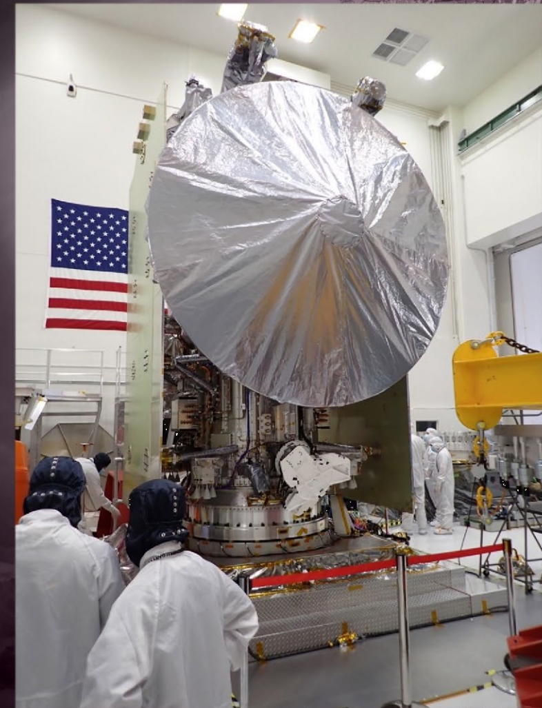
High-Gain Antenna after radome removal in cleaning orientation
