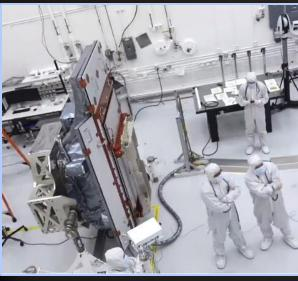
Roman WFI recently underwent vibration and acoustics testing and successfully completed its second and final thermal vacuum test in May.
