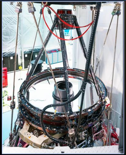
The entire optics system for Roman consists of 10 mirrors, including the 7.9-foot (2.4 meter) primary mirror seen at the base of this image called the Imaging Optical Assembly (IOA). Engineers recently integrated and tested the IOA at L3Harris Technologies in Rochester, NY. Credit: NASA/Chris Gunn
