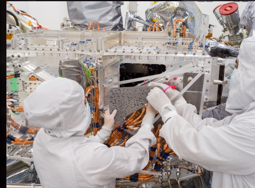
Europa Clipper vault plate installation at JPL
