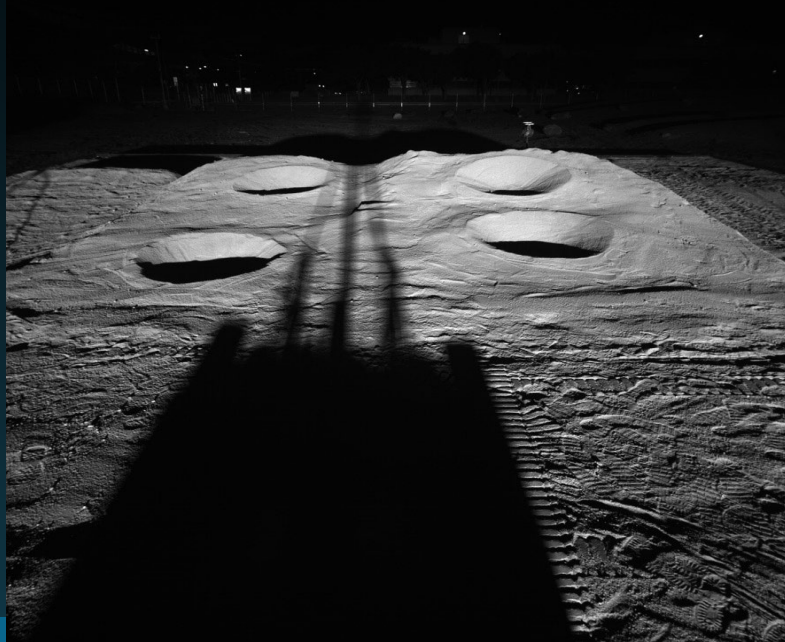
Engineering Unit Rover NavCam view with Sun Simulator from behind
