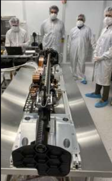
Subsurface excavation TRIDENT Drill
