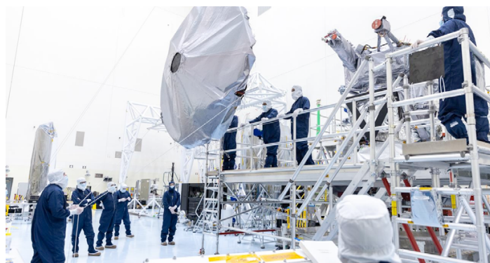
Technicians at NASA's Kennedy Space Center prepare to install Europa Clipper's 10-foot (3-meter) high-gain antenna. Credit: NASA/Kim Shiflett
