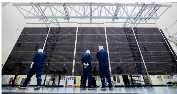
Technicians at NASA's Kennedy Space Center examine one of Europa Clipper's two five-panel solar arrays. Credit: NASA/Ben Smegelsky
