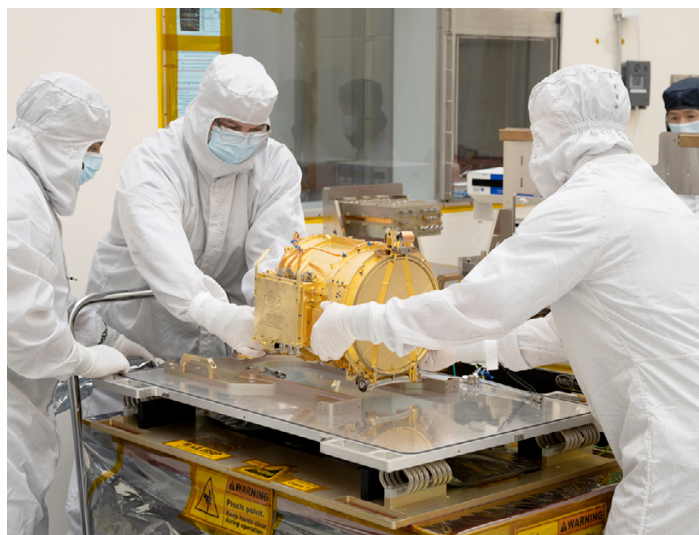
Technicians prepare Europa Clipper's dust-analyzing instrument for installation on the spacecraft. Europa Clipper carries a suite of nine instruments and a gravity experiment. Credit: NASA/JPL-Caltech | Full Image
